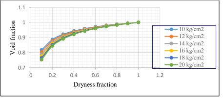
Figure 5. Void fraction Vs Dryness fraction
