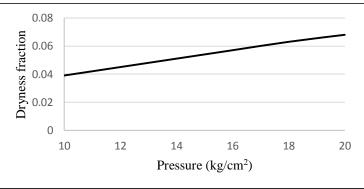
Figure 6. Effect of pressure on acceptable dryness fraction
