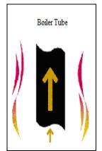
Figure 2.Riser fluid flow
