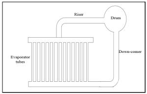
Figure 1.Circulation circuit of boiler
