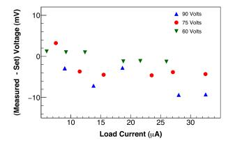
FIG. 5. Load regulation characteristics of one of the PPS channels.
