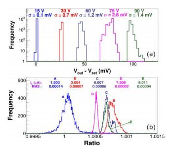
FIG. 6. Results of PPS stability at different applied voltages; (a) distribution of difference between applied and measured voltage. An offset of 25 mV was introduced between successive distribution for better visibility. (b) Distribution of ratio of PPS current to *true* current.
