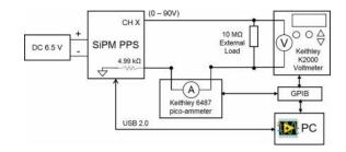
FIG. 3. Block diagram of experimental setup for calibration of the PPS system.
