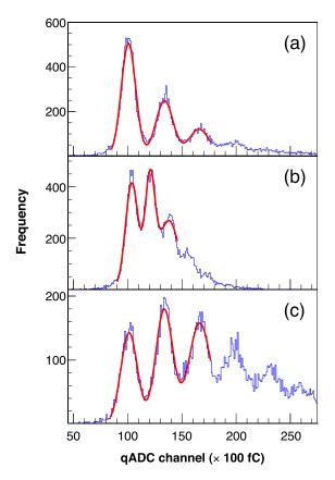
FIG. 8. Distribution of SiPM response to pulsed laser light at (a)  $20^{\circ}$ C, (b) at  $34.5^{\circ}$ C without temperature compensation, and (c) at  $34.5^{\circ}$ C with temperature compensation. The distributions have been fitted with multi-peak Gaussian function.
