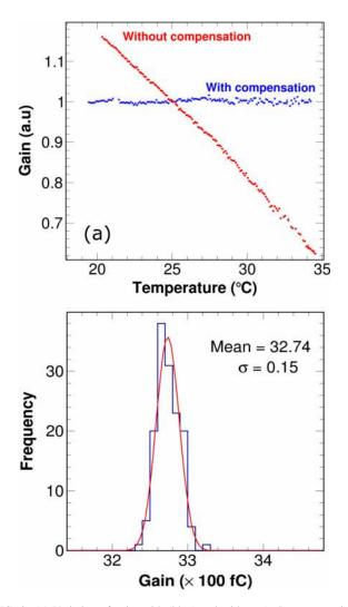
FIG. 9. (a) Variation of gain, with (blue) and without (red) compensation algorithm. Gain was normalized to the value at 25 °C. (b) Distribution of SiPM gain over a temperature range of 15 °C with temperature compensation enabled. A gain stability of 0.5% was achieved.
