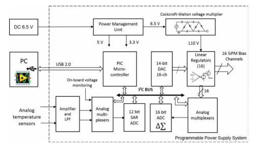
FIG. 1. Block diagram of multi-channel programmable power supply (PPS) system.
