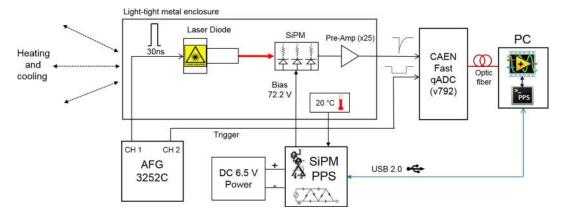
FIG. 7. Experimental setup used to record SiPM response to pulsed laser light.
