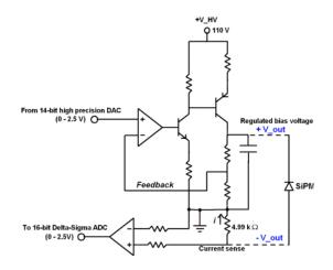
FIG. 2. Schematic of the programmable linear regulator with current sensing mechanism for one channel.
