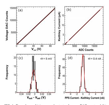
FIG. 4. Dependence of (a) measured output voltage on DAC count and (b) ADC counts on *true* load current. Linear fits in sub-divided ranges are used to obtain calibration parameters. (c) Distribution of difference between set voltage ( $V_{set}$ ) and measured output voltage ( $V_{out}$ ) voltage obtained in the range of 0-90 V. (d) Distribution of difference between load current measured with PPS system and *true* current measured by Keithley pico-ammeter.
