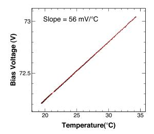
FIG. 10. Variation of bias voltage generated by SiPM PPS as a function of temperature. The set temperature coefficient was reproduced in the data.
