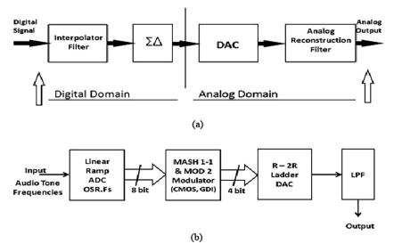
Fig. 1. (a) Block Diagram of Delta Sigma DAC, (b) Implemented Block Diagram of Delta Sigma DAC.
