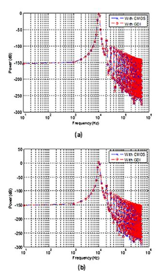
**Fig. 9.** (a) Output Power Spectrum of 10 kHz CMOS and GDI based MASH 1-1 with DC removed, (b) Output Power Spectrum of 10 kHz CMOS and GDI based MOD 2 with DC removed.
