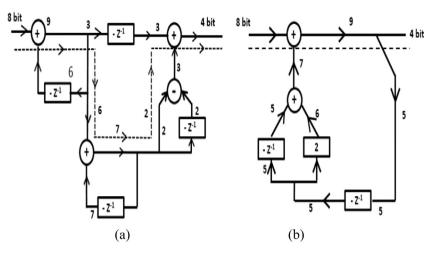
Fig. 8. (a) Path for calculating propagation delay of MASH 1-1, (b) Path for calculating propagation delay of MOD 2.
