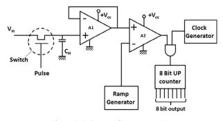
Fig. 4. Block diagram of Linear Ramp ADC.
