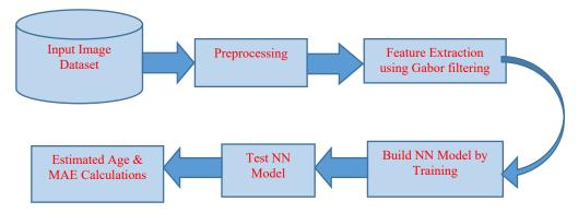
Fig. 1. Steps for age estimation using Neural Network
