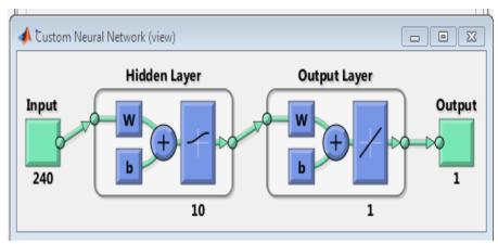
Fig. 5 Architecture of Neural Network
