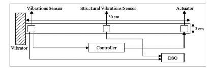
Fig. 2. Block Diagram of Experimental Setup.
