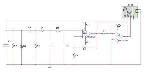
Fig. 5. Vibration Sensor Along with Inverter Circuit.
