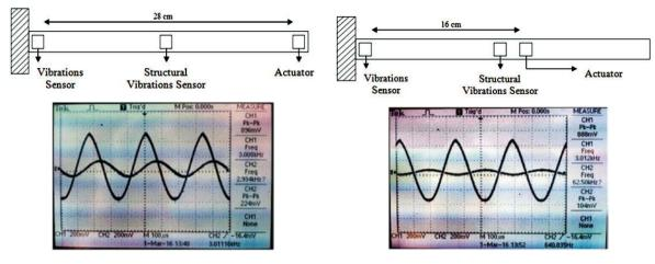
Fig. 7. Output of the System for D = 28 cm.
