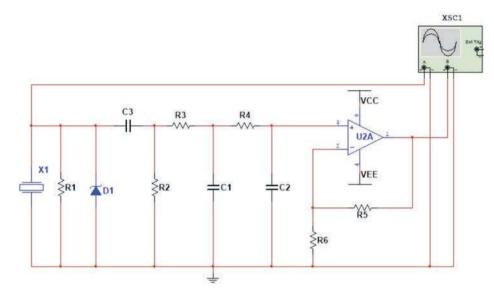
Fig. 4. Vibration Sensor Circuit.
