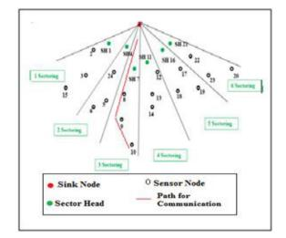
**Figure 6.** Static sectoring scheme for reliable data communication.
