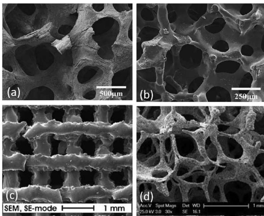
**Fig. 1.** SEM images of (a) human trabecular bone [19] (b) 13-93 bioactive glass scaffold [19] (c) Ti-6Al-4V structure [44] (d) TiNbZr scaffold [26].
